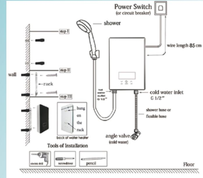
1. Drill into the wall with electric drill;
